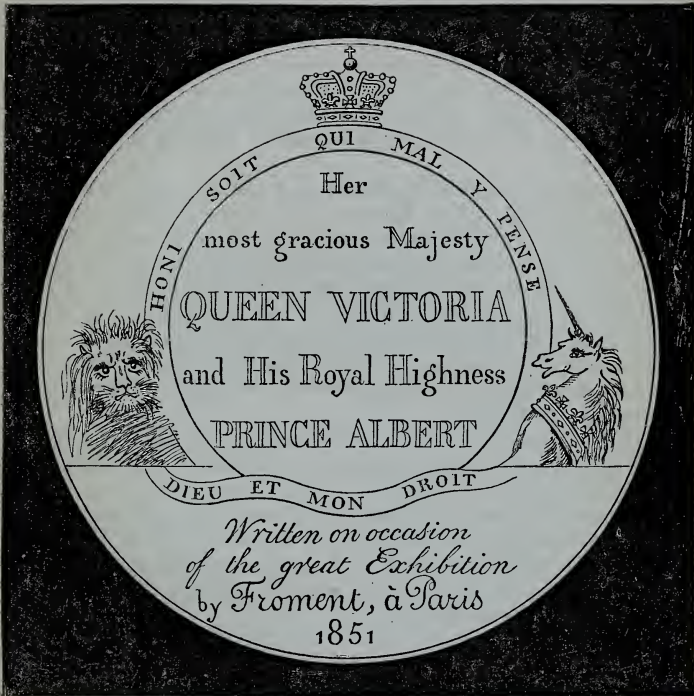
Fig. 8.—Appearance as seen in the field of the Microscope the outer circle being only 1-30th of an inch in diameter.
